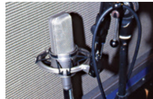
figure-of-eight frequency response: 20–18,000 Hz
